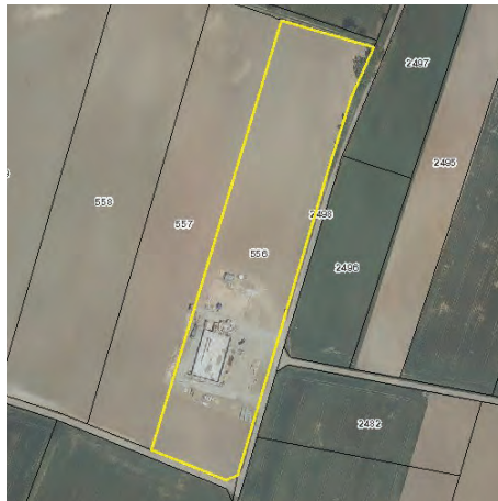
Figure 3. Example of a building right in the Austrian cadastral map. Source: BEV, Federal Office of Metrology and Surveying, Republic of Austria.
