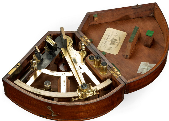
Slika 3: Sekstant znamke Dolland. S takšnim sekstantom je Thompson izvajal svoje astronomske in geodetske meritve. Vir slike: https://www.1stdibs.com/furniture/more-furniture-collectibles/collectibles-curiosities/scientific-instruments/brass-sextant-william-dolland/id-f_29626112/ .
